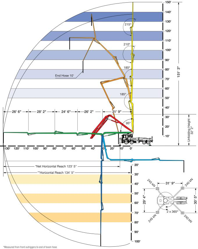
\*\*Measured from center of turret to end of boom hose
