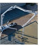
Schwing's 5-section Hyper Extension Roll and Fold® boom features extra articulation at every boom section including 215 degrees at the tip. Exceptional maneuverability and versatility comes with a compact travel position and low 32' 2" unfolding height. The generous 730 degree slewing range means the operator finishes faster for more jobs in a day.
