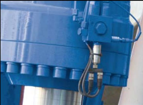
Sensors on the boom cylinders work with the Ergonic system to control Extended Range EBC.
