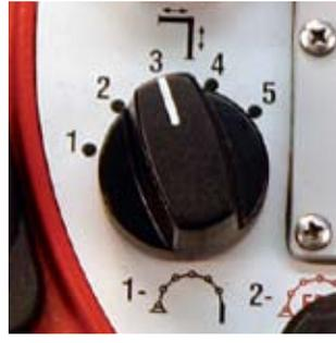
3 Semi-automatic folding in/out of the boom
